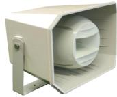
The MHE50T-EN5424 is a horn-type sound projector speaker. It combines acoustical performance of a sound projector with sound pressure of a horn loudspeaker . It allows to get a high public address sound quality together with a long range. Made out of ABS, it is weatherproof, shock and corrosion resistant. Its fixing device facilitates its orientation and ensures an easy and quick installation.
